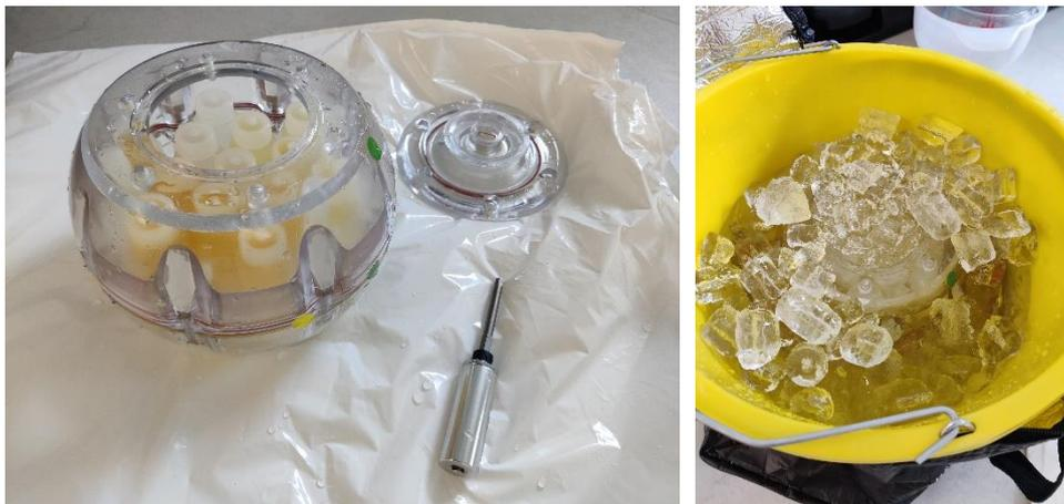
*Figure A2. The phantom is emptied by removing the end covers (left) and then submerged in a bucket filled with ice and chilled water for 15 minutes (right).*
