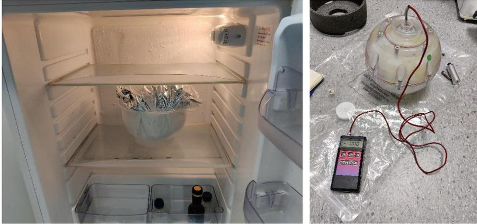
*Figure A3. Left: The phantom is left in the fridge for approximately 2 hours, wrapped in an insulating blanket. Right: Phantom temperature is measured through the fine fill port.*
