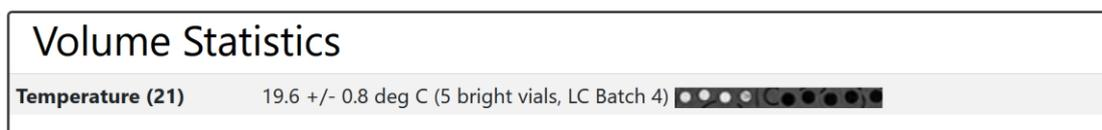
*Figure 18. Incorrect ROI placement for the LC Vials can lead to errors in the temperature measurement. The fifth vial is ‘dark’; however, the VOI is misplaced and therefore ‘bright’, increasing the reported temperature.*
