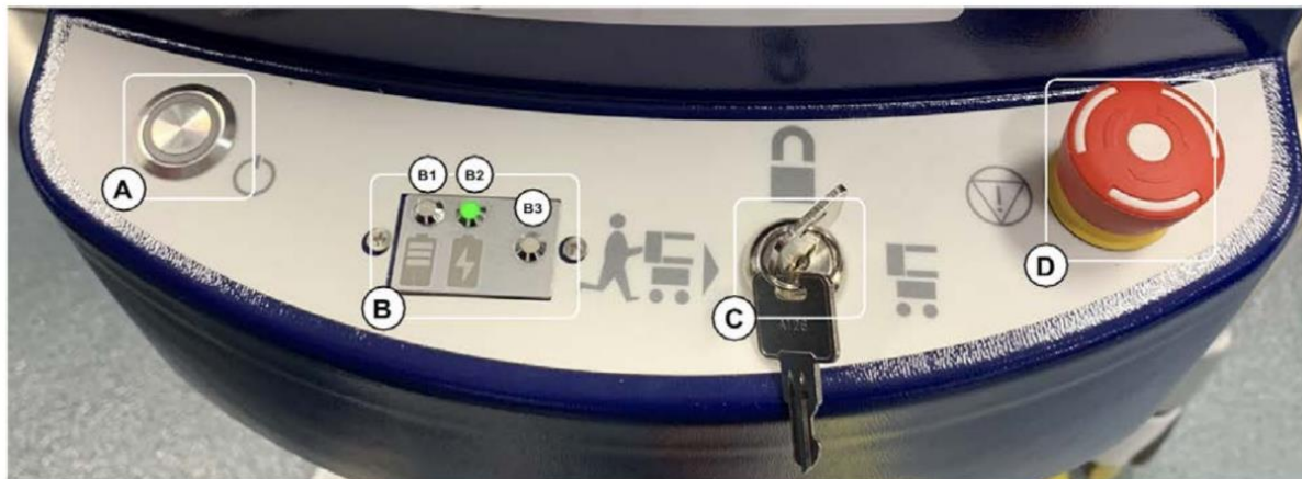
Figure 2: Control Panel - (A) Power Button, (B) Battery Indicators, (C) Mode Key Switch, and (D) E-Stop
